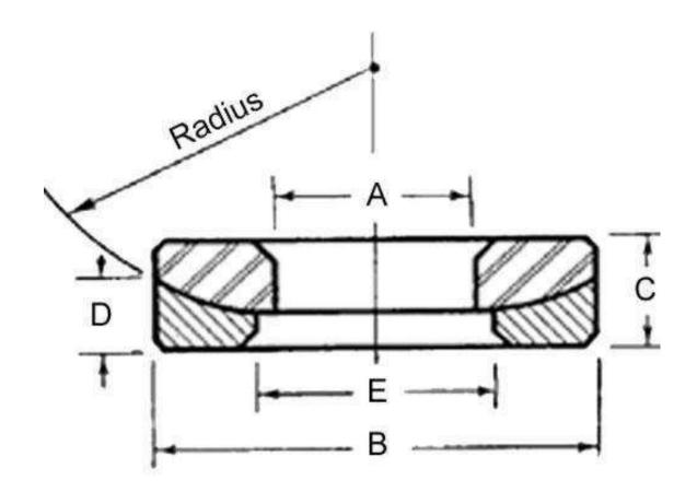
Washers - Self Aligning - Sets - Stainless Steel
